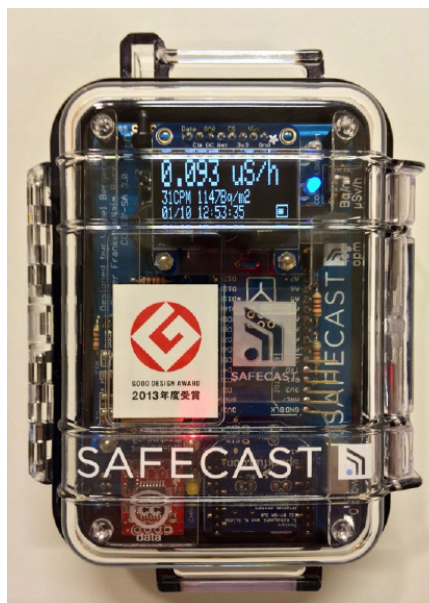
The bGeigie Nano is the current workhorse of Safecast's radiation measurement efforts.
