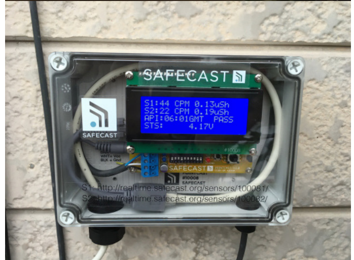
Pointcast hardware elements: Top: Medcom Hawk detector; Bottom: Pointcast control and communication unit.
